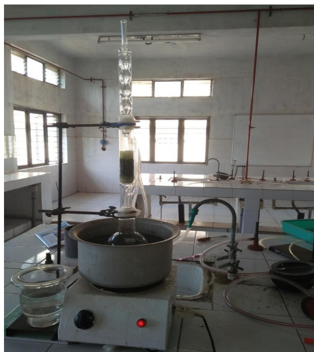
Fig 3: Soxhlet extract of plant material
