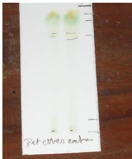
Fig 6: TLC Profile of the Pet ether extract of P. guajava leaf. Solvent system: benzene: chloroform:ethyl acetate (4:3:3)
